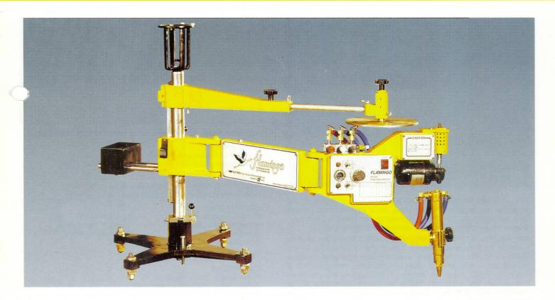
lamingo is a small portable radial arm oxygen cutting machine. Being small in size and light in weight, the machine can be easily carried to the worksite and placed directly on the plate to be cut. As the machine is mounted on four ball castors, it can be moved about on the plate as required.
